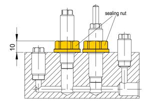
Accessories: Sealing nut (tightening torque max. 25 Nm) Order No: 7012-056
