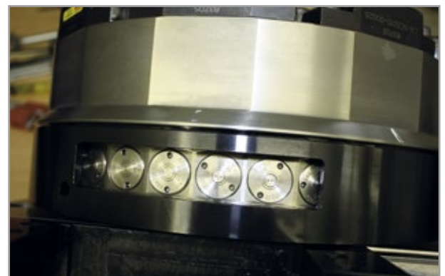
The revolver with a total of 36 coupling nipples.
