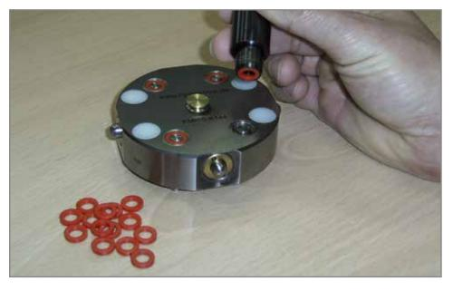
Mounting tool with inserted system seal prior to pressing into the coupling mechanism.
