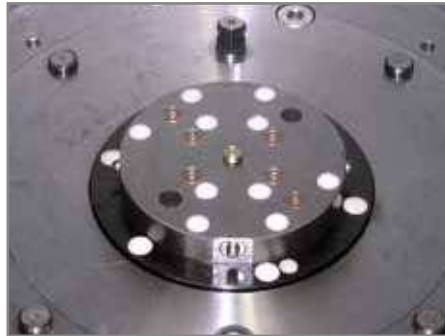
Docking system in the loading and unloading station of a machine tool. In order to allow 360° rotation of the hydraulic clamping fixture the system is equipped with a rotary coupling.
